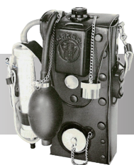
Riken type 18 gas detector (developed in 1952)
